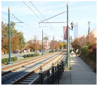
Figure 1-14. Fixed-Termination Single Contact Wire Sharing a Pole with Street Lights
