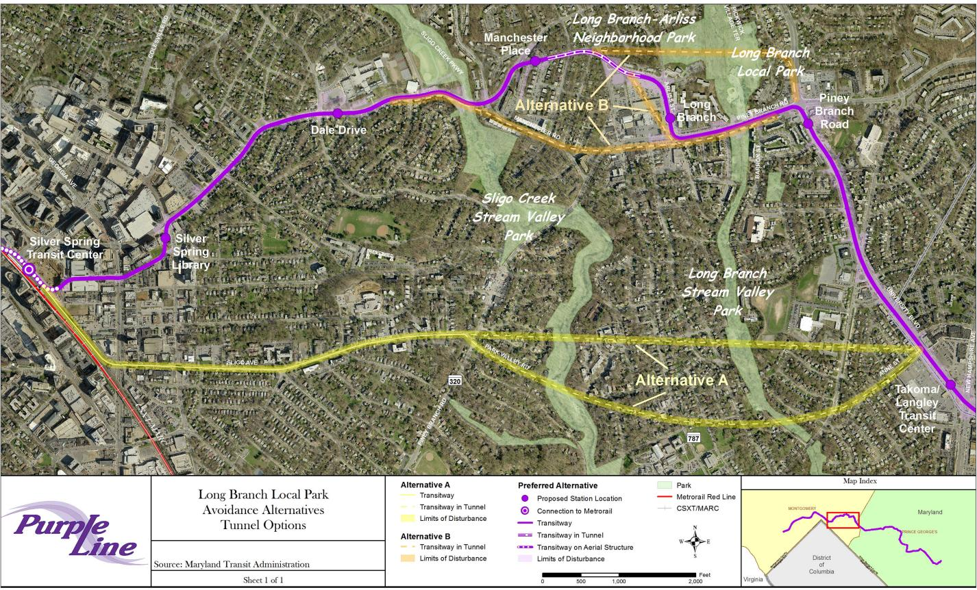
Figure 1-23. Long Branch Local Park Avoidance Alternatives—Tunnel Options
